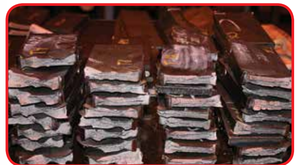
Fracture surfaces of tested specimens
